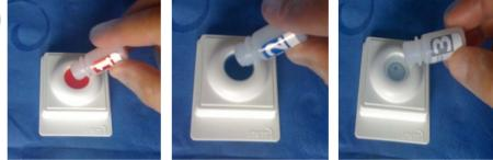
Pour the entire contents (1 then 2 then 3) to the center of the membrane unit well. Wait for total absorbtion of the sample before pouring the following solutions. Read the result immediatly.
